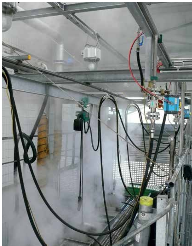
J D Neuhaus air operated hoist in operation for precise handling of pressure injection head during tank cleaning operation
